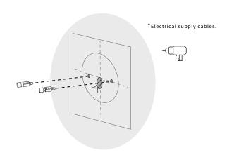
Mount the light fixture on the wall.
