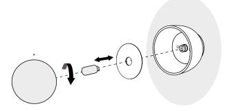
$^{\star}$ Align the glass diffuser and screw gently to avoid jamming.
