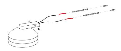
2 Connect the cables +with+&-with-through the thermofit.
