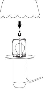
After placing the metal lamp shade, connect the lamp to the power supply.
