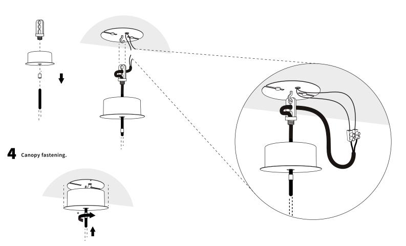
${}^{\star}\mathsf{Screw}$  fastener lightly until the canopy is secure.
