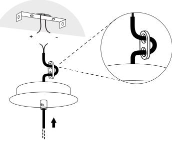
3 Connect the wires through the connector.
