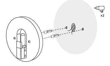
**2** Connect the wires through the connector.
