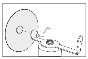
\*Place the washer between the screw and the holder to adjust the assembly.
