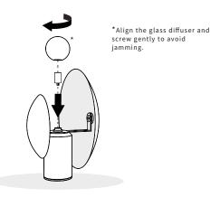
Place the holder on top of the base and fix it with the ring.
