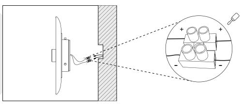
4 Fix the lamp to the wall and place the LED Bulb.
