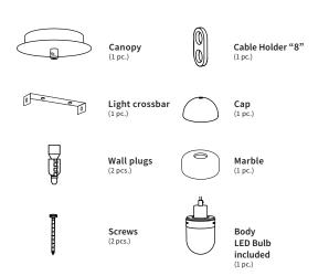
Cut the cable to the desired lenght. Place the wall plugs and fix the light crossbar to the ceiling.
