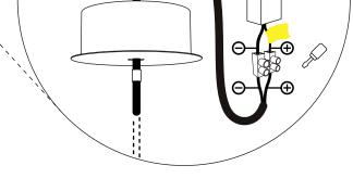
Connection of cables from lamp to Driver:
