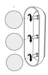
\*Align the glass diffuser and screw gently to avoid jamming.
