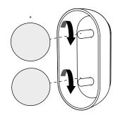
\*Align the glass diffuser and screw gently to avoid jamming.
